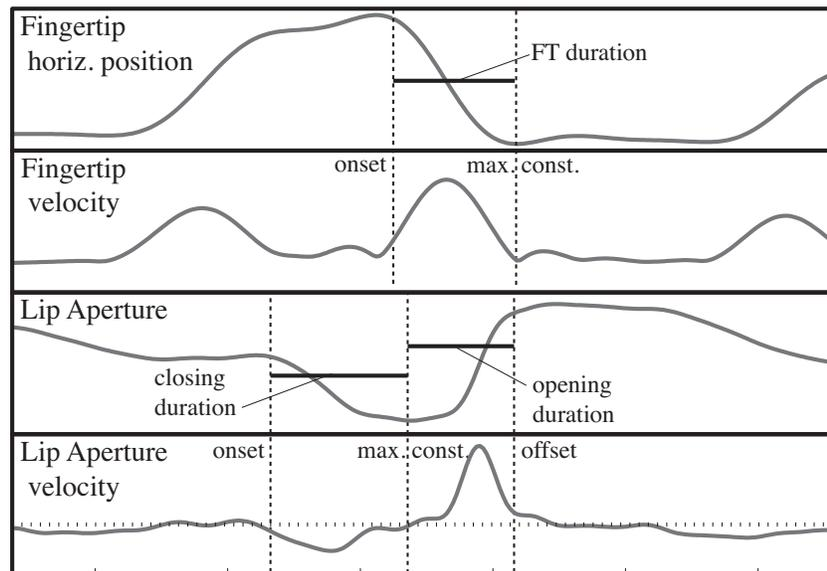
**Figure 1.** Labeling and measurements made from articulatory data. Location of relevant articulatory events is based on the velocity signal for both lip and finger movements; horizontal motion of the finger tip shown for illustration only. Both opening and closing durations of syllable-initial /m/ were measured.
