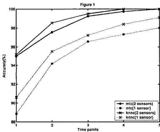
Figure1: Classification performance for inter-node collaboration between two sensors (solid lines) for 2 different classifier types; Maximum Likelihood (mlc) and kNearest (knnc) plotted against duration of sampling.
