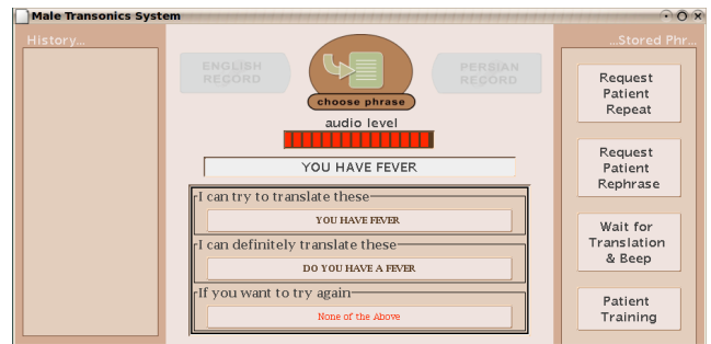
Fig. 2. Example image of the system’s Graphical User Interface (GUI). After speaking, the English speaker (doctor) can choose one of up to five translation candidates presented onscreen. Section 1 shows the SMT option E_1 labeled with “I can try to translate”, while the CCMT options E_i \forall i \in \{2, 3, 4, 5\} are labeled “I can definitely translate these”
