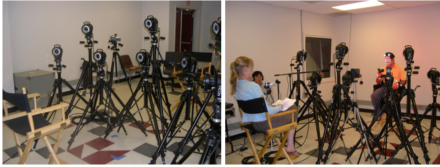
Figure 3. VICON motion capture system with 8 cameras. The subject with the markers sat in the middle of the room, with the cameras directed to him/her. The subject without the markers sat outside the field of view of the VICON cameras, facing the subject with markers.
