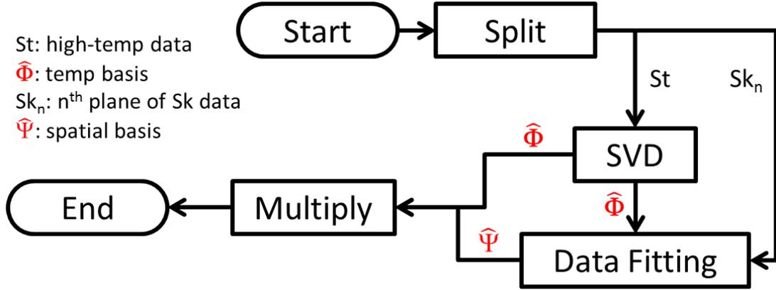
Figure 2: Diagram of PS model reconstruction from the data acquired using sampling scheme in Figure 1. The PS model is applied pairwise to the frequently sampled plane and one of the remaining planes.
