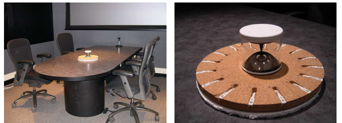
Fig. 1. On the left is the instrumented conference room and on the right is the 16-microphone array with the omni-directional camera above it.
