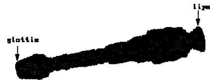
Figure 7: Tube model for subject MI's /a/ with an extrapolated 1mm mesh thickness used in FTD simulations.
